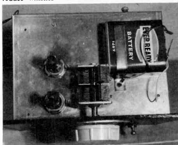
Top view of completed converter.
